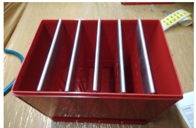
Fig. (b) Placement Of Aluminum Strip on Partition wall
